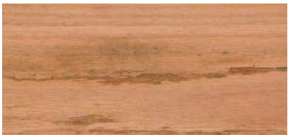
SHAKE A separation between the annual growth rings.
